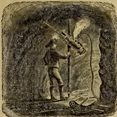
VIEW OF DRILL ATTACHED TO COLUMN, AS USED WITH COMPRESSED AIR OR STEAM, WHEN PRACTICABLE.
